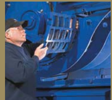
Grate changes can be made quickly. Thanks to our patented multiple grate system, it's easy to produce a range of high-quality products.
