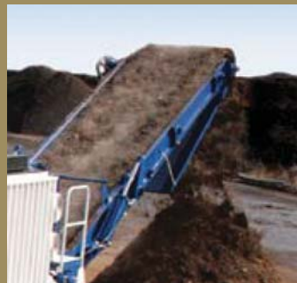
Wide discharge conveyor with variable speeds and magnetic headroll allows effective metal separation and high capacity production.
