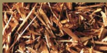
Biofuel from scrap board processed with a 4-inch grate.
